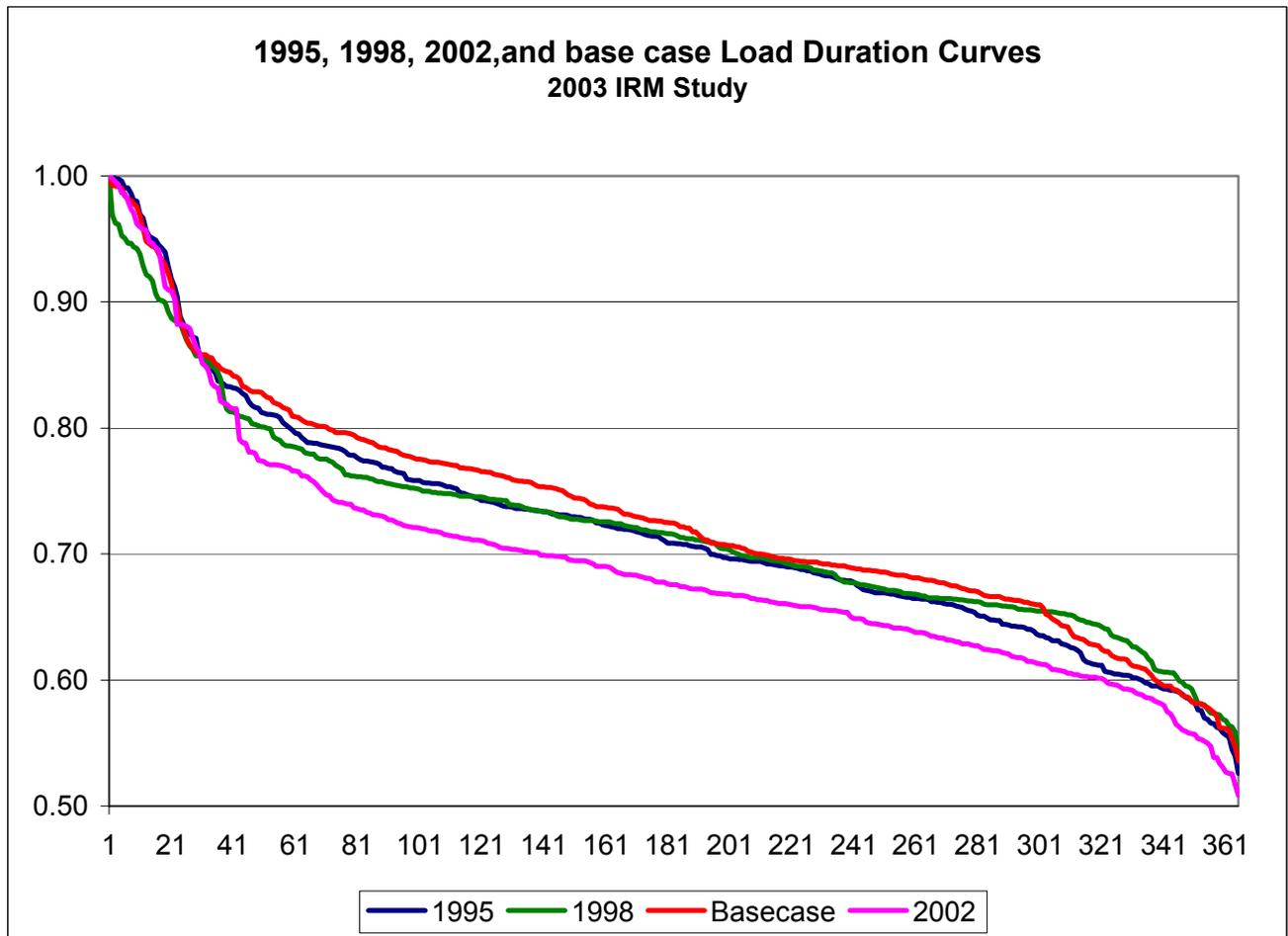
The load shape for a zone that is input into MARS is an hourly aggregate of sub-zone loads. Sub-zone loads in NYCA are developed by applying appropriate weights to the Transmission District load shapes.
