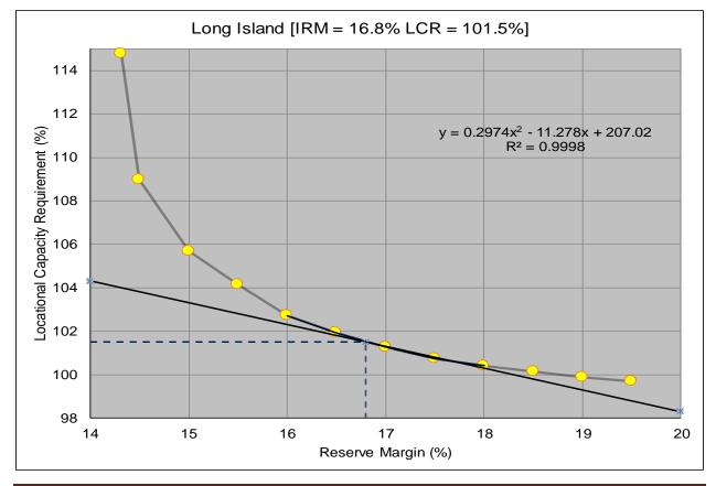
NYCA Installed Capacity Requirement for the Period May 2019 through April 2020
