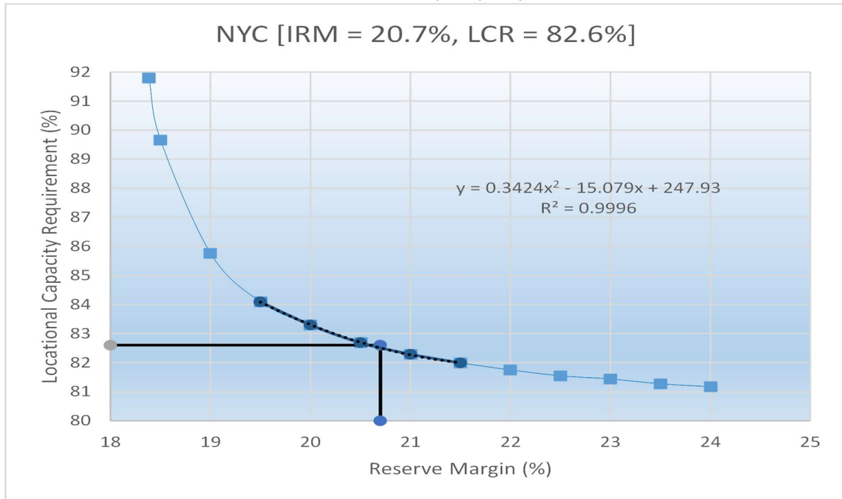
TO BE UPDATED Figure 3-2 Relationship Between NYCA IRM and Corresponding Initial Locational Capacity Requirements
