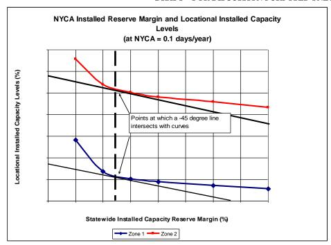
Figure 3-2: Unified Curve and IRM Anchor Point
