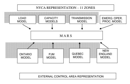
Figure 2-1: Relationship between MARS and the Models Used In the IRM Requirement Calculation Process
