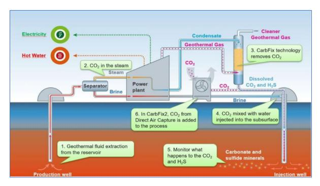
Through than energy produced from fossil fuels, geothermal plants emit some CO2, as well as the hydrogen sulfide contained in steam. The CO2 from the steam is captured and dissolved in large amounts of water. The fizzy water is pumped to the injection site and is pushed over a mile a deep into basaltic rock, where it solidifies to rock in about 2 years. Trapped in the rock, the CO2 cannot leak out of the ground and into the atmosphere.
