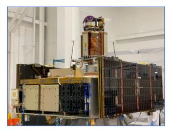
The prototype also beamed a tiny but detectable amount of energy to a receiver on top of their lab's building in Pasadena, Calif. The demonstration marks a first step in the wireless transfer of usable power from space to Earth — a power source that will be safer than direct sun rays, as the beam intensity is to be kept less than solar intensity on earth.
