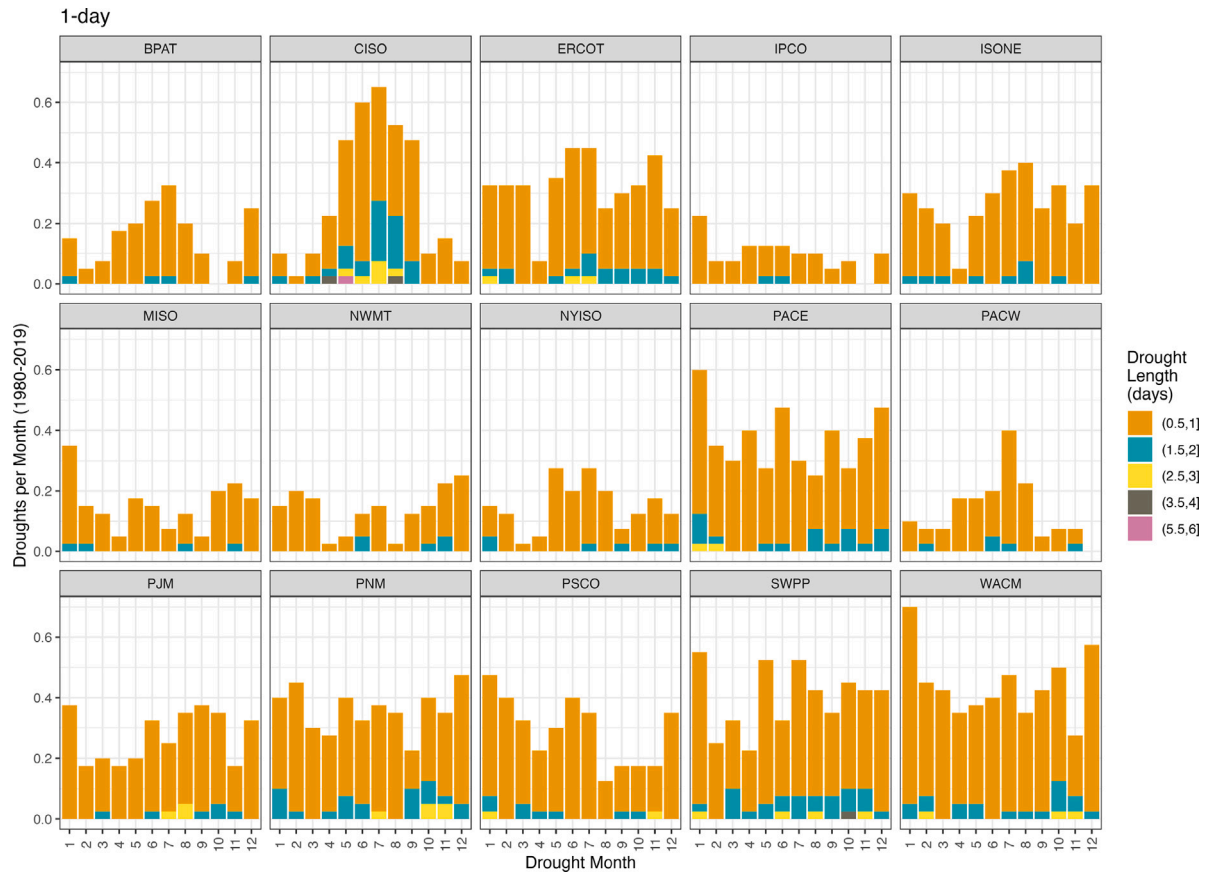
Fig. 5. Seasonal distributions of energy droughts. The bar heights indicate the frequency of droughts in a particular month (average number of droughts per year). The color indicates the drought duration.
