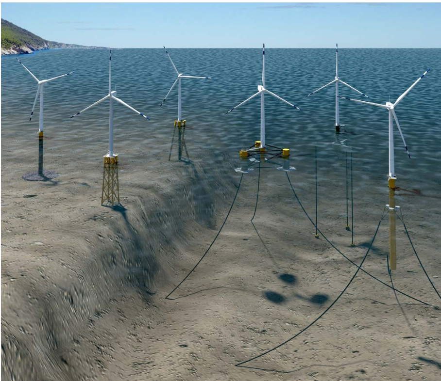
FIGURE 3. Offshore wind foundation types include, from left to right, monopile, jacket, twisted jacket, tension-leg floating platform, semi-submersible platform, and spar buoy. Illustration by Josh Bauer, National Renewable Energy Laboratory
