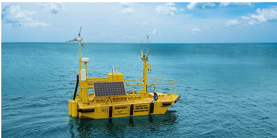
FIGURE 5. The photo shows the Pacific Northwest National Laboratory WindSentinel™ lidar buoy (manufactured by AXYS Technologies). The schematic drawings and numbered table provide technical specifications for the buoy ( https://www.pnnl.gov/projects/lidar-buoy-program/technical-specifications ).
