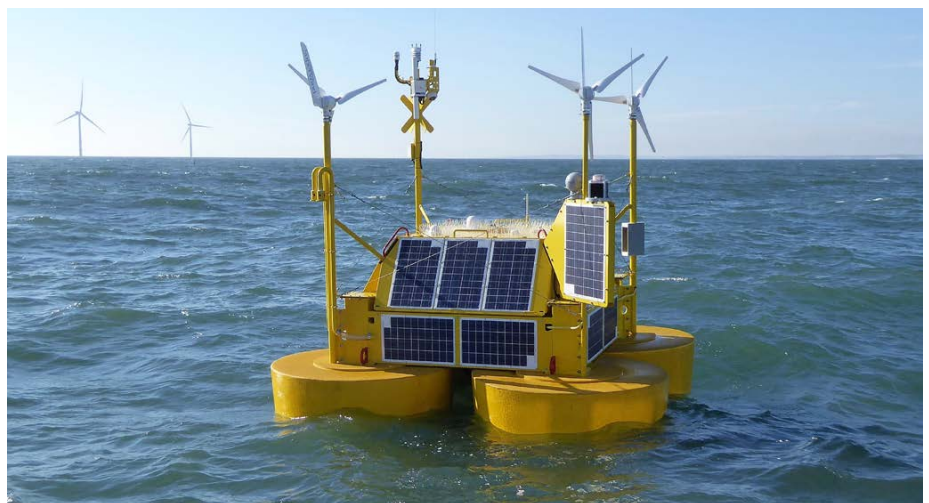
FIGURE 2. In 2019, the New York State Energy Research and Development Authority commissioned the deployment of two floating lidar buoys in the New York Bight. These buoy-based lidars provided nearly three years of physical metocean parameters to facilitate offshore wind development within the region. Parameters include multi-level wind speed and direction, wave, and current measurements, as well as other environmental and wildlife data. Courtesy of New York State Energy Research and Development Authority, https://oswbuoysny.resourcepanorama.dnvgl.com/overview
