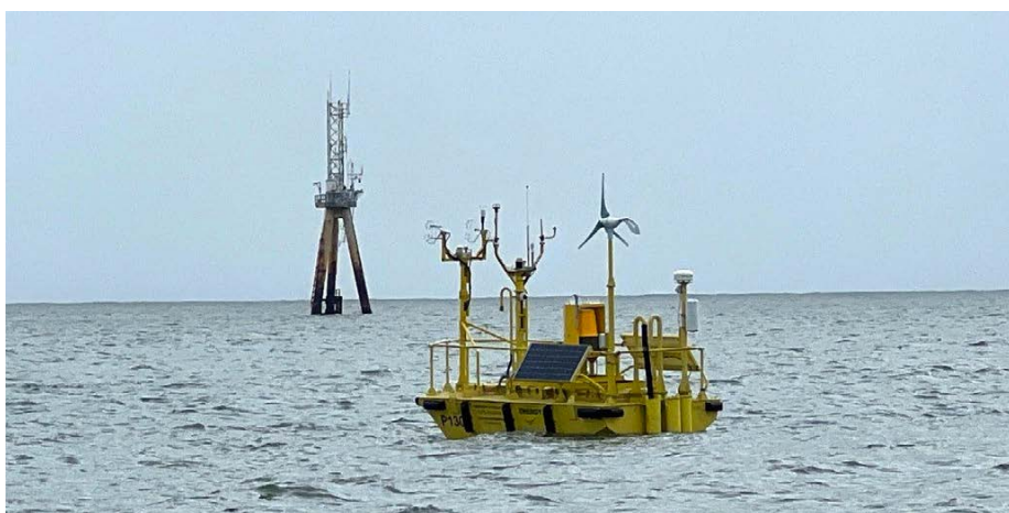
FIGURE 6. The Pacific Northwest National Laboratory lidar buoy newly equipped with a flux measurement package is shown deployed in the vicinity of the Air-Sea Interaction Tower (ASIT) near Martha's Vineyard. Package measurements include fluxes of moisture, momentum, and buoyancy. Photo courtesy of Pacific Northwest National Laboratory
